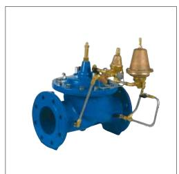
• It prevents from overflowing and maintains a constant level in the tank thanks to the pilot and guarantees a minimum upstream pressure.
