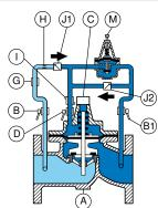
In case of down-stream overpressure, the check valve J2 canalizes the overpressure to the upper chamber and the check valve J1 prevents the overpressure from passing upstream. The valve A closes and stops any backpressure up-stream.
